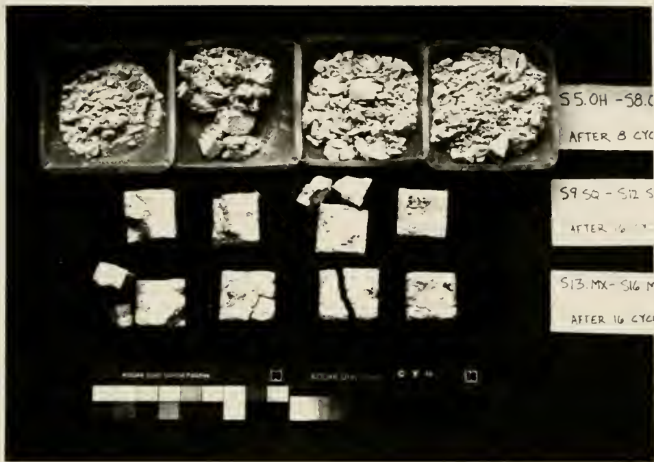
Figure 2.12 Appearance of facsimiles S5.OH - S8.OH after 8 cycles of salt crystallization, and appearance of facsimiles S9.SQ - S12.SQ and S13.MX - S16.MX after 16 cycles of salt crystallization.
